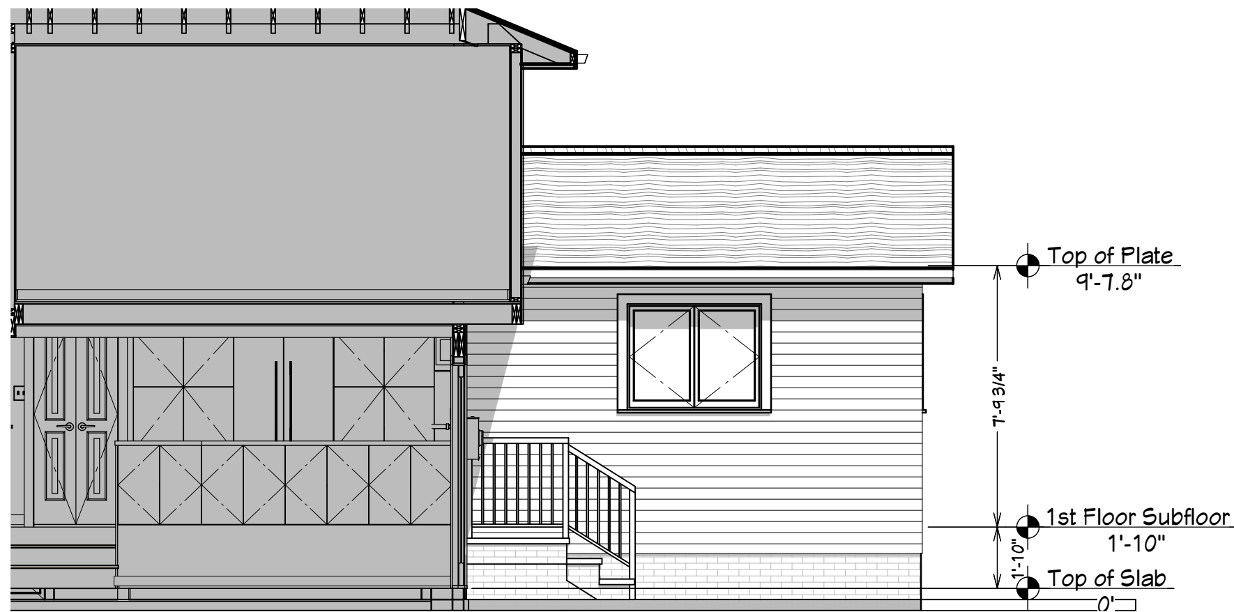
2 Right Elevation - Kitchen Addition A-5 1/4 in = 1 ft
