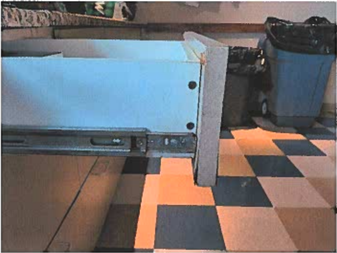
Drawer laminate separation
