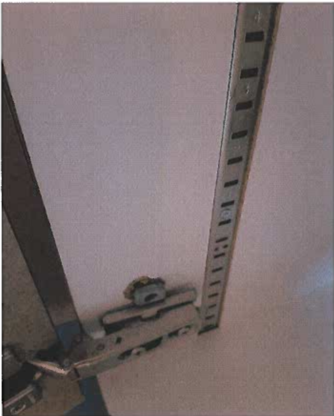
Hinge screw pulled out of pressed wood cabinet.
